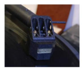
to access the bolt holes. You're advised not to overtighten the nuts—doing so can split the hardwood body.
